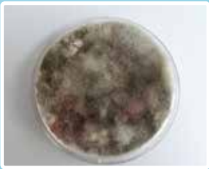
Agar plate sample showing mould growth from Cooling Coil
